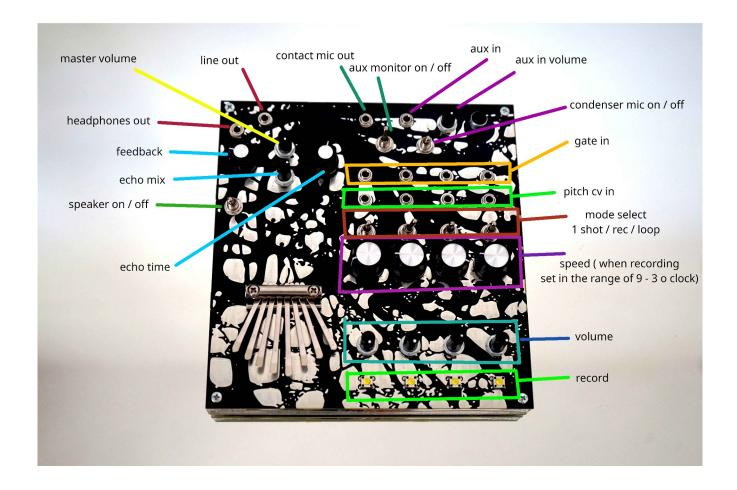
La Madrugada is a 4 track lo fi sample recorder with 2 built in microphones – 1 contact mic and 1 electret condenser mic. You can also record aux sources.
